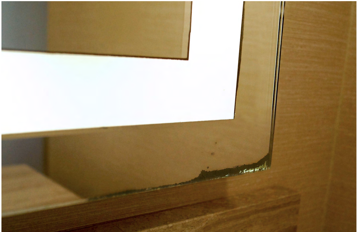
Competitive Mirror Black Edge Corrosion
